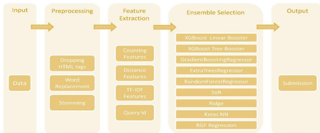
FIGURE 4.1 Flow Chart of the Work The measurement of the separate model and the ensemble model[2]
